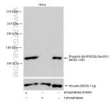
Non-treated HeLa cells, phosphatase inhibitor treated HeLa cells and  $\lambda$  phosphatase treated HeLa cells were subjected to SDS PAGE followed by western blot with 84563-1-RR (Phospho-SH3PKD2B (Ser291) antibody) at dilution of 1:2000 incubated at room temperature for 1.5 hours. The membrane was stripped and re-blotted with Vinculin (66305-1-Ig) antibody as a loading control.
