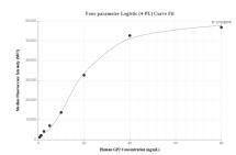
Cytometric bead array standard curve of MP01513-1, GP2 Recombinant Matched Antibody Pair, PBS Only. Capture antibody: 84728-1-PBS. Detection antibody: 84728-3-PBS. Standard: Eg2446. Range: 0.625-80 ng/mL
