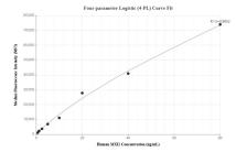
Cytometric bead array standard curve of MP01509-1, MXI1 Recombinant Matched Antibody Pair, PBS Only. Capture antibody: 84733-2-PBS. Detection antibody: 84733-4-PBS. Standard: Ag3024. Range: 0.625-80 ng/mL
