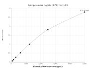
Sandwich ELISA standard curve of MP01720-3, Human RAD50 Recombinant Matched Antibody Pair - PBS only. 84969-1-PBS was coated to a plate as the capture antibody and incubated with serial dilutions of standard Ag29949, 84969-2-PBS was HRP conjugated as the detection antibody. Range: 78.1-5000 pg/mL
