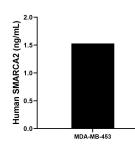
The mean SMARCA2 concentration was determined to be 1.53 ng/mL in MDA-MB-453 cell extract based on a 1.5 mg/mL extract load.
