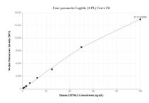
Cytometric bead array standard curve of MP01862-2, ZFP36L2 Recombinant Matched Antibody Pair, PBS Only. Capture antibody: 85154-2-PBS. Detection antibody: 85154-1-PBS. Standard: Ag13515. Range: 0.781-100 ng/mL
