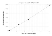
Cytometric bead array standard curve of MP02037-1, KTN1 Recombinant Matched Antibody Pair, PBS Only. Capture antibody: 85681-3-PBS. Detection antibody: 85681-2-PBS. Standard: Ag13854. Range: 1.563-100 ng/mL
