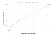
Cytometric bead array standard curve of MP02183-1, TAF 1B Recombinant Matched Antibody Pair, PBS Only. Capture antibody: 85885-1-PBS. Detection antibody: 85885-2-PBS. Standard: Ag38211. Range: 0.781-100 ng/mL
