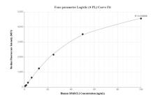
Cytometric bead array standard curve of MP02200-1, SPARCL1 Recombinant Matched Antibody Pair, PBS Only. Capture antibody: 85906-3-PBS. Detection antibody: 85906-2-PBS. Standard: Eg2837. Range: 0.781-100 ng/mL.
