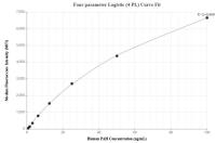
Cytometric bead array standard curve of MP02346-1, PAH Recombinant Matched Antibody Pair, PBS Only. Capture antibody: 86231-2-PBS. Detection antibody: 86231-1-PBS. Standard: Ag9541. Range: 0.781-100 ng/mL
