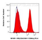
1x10^6 mouse splenocytes were surface stained with 0.25 ug Anti-Mouse CEACAM1/CD66a Rabbit Recombinant Antibody (98185-1-RR, Clone: 241856H5) (red) or 0.25 ug Isotype Control (blue), and PF-Conjugated Goat Anti-Rabbit IgG(H+L). Cells were co-stained with Coralite® Plus 647 Anti-Mouse CD45R. Cells were incubated with FC Receptor Block prior to staining. Cells were not fixed.
