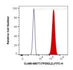
1X10^6 HeLa cells were intracellularly stained with 0.4 ug CoraLite® Plus 488 Anti-Human TPD52L2 (CL488-68077, Clone:3B3C6) (red), or 0.4 ug Mouse IgG2b Isotype Control (CL488-66360-3, Clone: K11B8C4B5) (blue). Cells were fixed with 4% PFA and permeabilized with Flow Cytometry Perm Buffer (PF00011-C).
