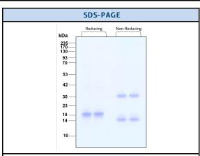
Purity of recombinant human IL-28A was determined by SDS- polyacrylamide gel electrophoresis. The protein was resolved in an SDS- polyacrylamide gel in reducing and non-reducing conditions and stained using Coomassie blue.
