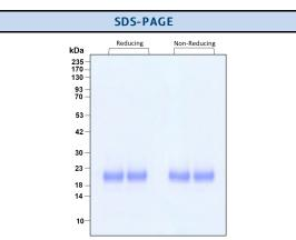
Purity of GMP-grade recombinant human IL-1 alpha was determined by SDS- polyacrylamide gel electrophoresis. The protein was resolved in an SDS- polyacrylamide gel in reducing and non-reducing conditions and stained using Coomassie blue.
