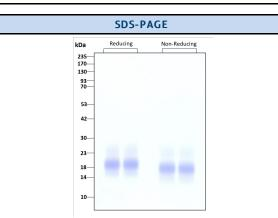
Purity of recombinant human IL-15 was determined by SDS- polyacrylamide gel electrophoresis. The protein was resolved in an SDS- polyacrylamide gel in reducing and non-reducing conditions and stained using Coomassie blue.
