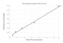
Cytometric bead array standard curve of MP00001-2, AFP Recombinant Matched Antibody Pair, PBS Only. Capture antibody: 82982-3-PBS. Detection antibody: 82982-2-PBS. Standard: Eg0539. Range: 1.25-20 ng/mL
