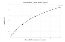
Sandwich ELISA standard curve of MP00006-3, PDGFR beta/CD140b Recombinant Matched Antibody Pair, PBS Only. Capture antibody: 82943-6-PBS. Detection antibody: 82943-3-PBS. Standard: Eg0147. Range: 0.156-10 ng/mL
