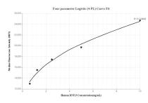
Cytometric bead array standard curve of MP00008-1, RNF 13 Recombinant Matched Antibody Pair, PBS Only. Capture antibody: 83066-3-PBS. Detection antibody: 83066-2-PBS. Standard: Ag8987. Range: 0.625-10 ng/mL
