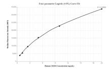
Cytometric bead array standard curve of MP00030-1, CD200 Recombinant Matched Antibody Pair - PBS only. Capture antibody: 83051-3-PBS. Detection antibody: 83051-4-PBS. Standard: Eg0006. Range: 0.625-20 ng/mL
