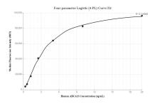
Cytometric bead array standard curve of MP00084-1, ABCA 13 Recombinant Matched Antibody Pair, PBS Only. Capture antibody: 83060-1-PBS. Detection antibody: 83060-2-PBS. Standard: SY00509. Range: 0.312-20 ng/mL
