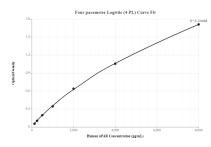
Sandwich ELISA standard curve of MP00129-1, uPAR/CD87 Recombinant Matched Antibody Pair, PBS Only. Capture antibody: 82953-2-PBS. Detection antibody: 82953-3-PBS. Standard: Ag28056. Range: 125-8000 pg/mL
