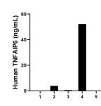
Sandwich ELISA standard curve of MP00218-3, Human TSG-6 Recombinant Matched Antibody Pair - PBS only. 83163-4-PBS was coated to a plate as the capture antibody and incubated with serial dilutions of standard Ag3885. 83163-3-PBS was HRP conjugated as the detection antibody. Range: 0.313-20 ng/mL
