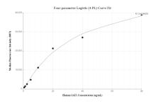
Cytometric bead array standard curve of MP00344-2, SAT1 Recombinant Matched Antibody Pair, PBS Only. Capture antibody: 83319-3-PBS. Detection antibody: 83319-1-PBS. Standard: Ag1154. Range: 0.625-80 ng/mL
