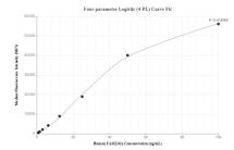
Cytometric bead array standard curve of MP00477-1, FAM116A Recombinant Matched Antibody Pair, PBS Only. Capture antibody: 83473-1-PBS. Detection antibody: 83473-3-PBS. Standard: Ag22052. Range: 0.78-100 ng/mL
