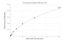
Cytometric bead array standard curve of MP00761-2, Granzyme B Recombinant Matched Antibody Pair, PBS Only. Capture antibody: 83763-2-PBS. Detection antibody: 83763-4-PBS. Standard: Eg0592. Range: 0.625-80 ng/mL
