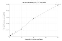
Cytometric bead array standard curve of MP00853-3, CHRNG Recombinant Matched Antibody Pair, PBS Only. Capture antibody: 83915-3-PBS. Detection antibody: 83915-4-PBS. Standard: Ag16489. Range: 1.25-80 ng/mL
