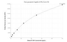
Cytometric bead array standard curve of MP01071-2, PC SK9 Recombinant Matched Antibody Pair, PBS Only. Capture antibody: 84172-1-PBS. Detection antibody: 84172-2-PBS. Standard: Eg0362. Range: 0.781-50 ng/mL
