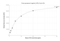
Cytometric bead array standard curve of MP01660-2, Complement factor D Recombinant Matched Antibody Pair, PBS Only. Capture antibody: 84851-2-PBS. Detection antibody: 84851-3-PBS. Standard: Eg1189. Range: 0.625-40 ng/mL
