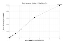
Cytometric bead array standard curve of MP01759-2, DOCK11 Recombinant Matched Antibody Pair, PBS Only. Capture antibody: 85022-3-PBS. Detection antibody: 85022-1-PBS. Standard: Ag35831. Range: 0.781-100 ng/mL.
