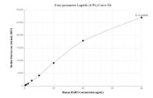
Cytometric bead array standard curve of MP02104-2, RLBP1 Recombinant Matched Antibody Pair, PBS Only. Capture antibody: 85697-4-PBS. Detection antibody: 85697-2-PBS. Standard: Ag7602. Range: 0.625-80 ng/mL
