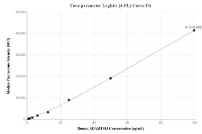
Cytometric bead array standard curve of MP02235-1, ADAMTS13 Recombinant Matched Antibody Pair, PBS Only. Capture antibody: 85974-2-PBS. Detection antibody: 85974-1-PBS. Standard: Eg2556. Range: 0.781-100 ng/mL.
