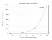
Cytometric bead array standard curve of MP50308-2, PM52 Monoclonal Matched Antibody Pair, PBS Only. Capture antibody: 68905-3-PBS. Detection antibody: 68905-4-PBS. Standard:Ag34237. Range: 1.563-100 ng/mL
