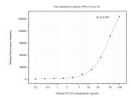
Cytometric bead array standard curve of MP50599-3, CCL24 Monoclonal Matched Antibody Pair, PBS Only. Capture antibody: 60443-3-PBS. Detection antibody: 60443-4-PBS. Standard:Eg0395. Range: 0.195-100 ng/ml.
