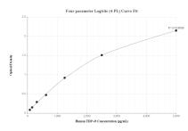
Sandwich ELISA standard curve of MP80000-1, TDP-43 Hybrid Matched Antibody Pair, PBS Only. Capture antibody: 60019-2-PBS. Detection antibody: 80001-1-PBS. Standard: Ag1833. Range: 78.1-5000 pg/mL
